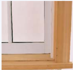
Window detail shown with standard 5/4 x 4 clear cedar exterior trim and standard 1-1/4" sill nosing profile. Optional 3/4" sill nosing extension past side trim. Clad simulated divided glass installed in the unit.
